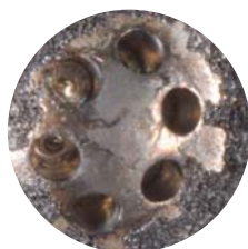
Injector after one P.i. treatment.
