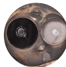
Cylinder head after one P.i. treatment.
